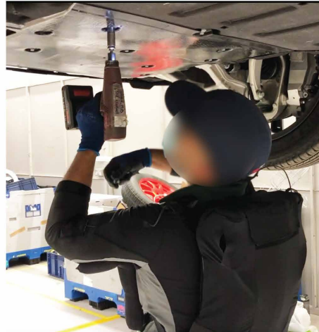
Fig. 7. Factory worker performing overhead tasks while assisted by the robot.
